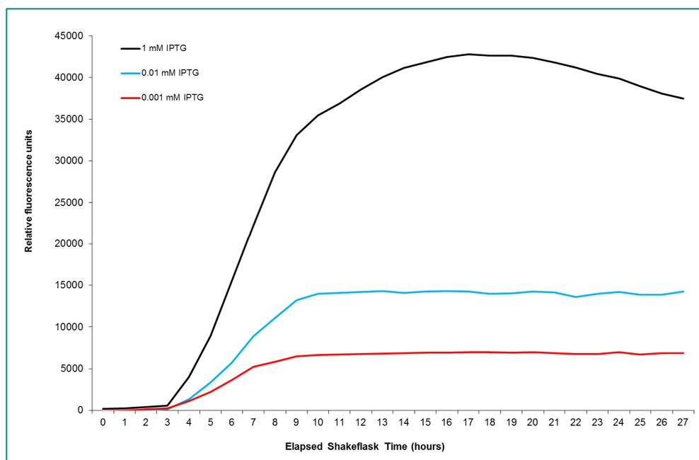
**Figure 2:** The effect of IPTG Concentration on GFP expression in pAVEway. IPTG Concentration is proportional to expression rate. This allows the production rate to be matched to protein folding and secretion rates. Induction takes place at 3 hours post inoculation. GFP Production monitored for further 24 hours.
